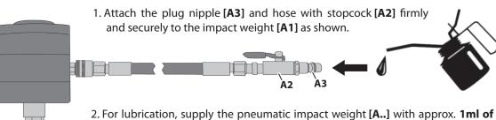
2. For lubrication, supply the pneumatic impact weight [A..] with approx. 1ml of pneumatic oil via the compressed air connection, then connect to a compressed air supply and briefly open the stopcock to allow the pneumatic oil to enter the interior.
