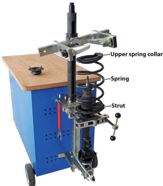
**📷 13:** Positioning the spring holder correctly on the spring collar.
