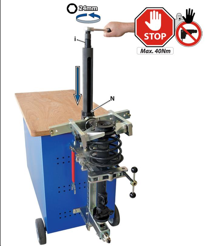
4) Turn the drive nut [i] clockwise until the spring holders [M] are positioned directly above the upper spring collar **📷7A**.
