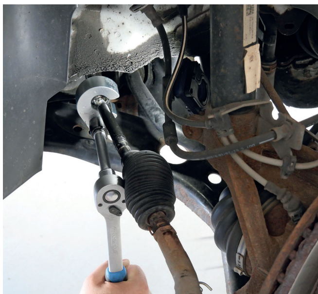
📷 3: Releasing / tightening the inner track rod.
