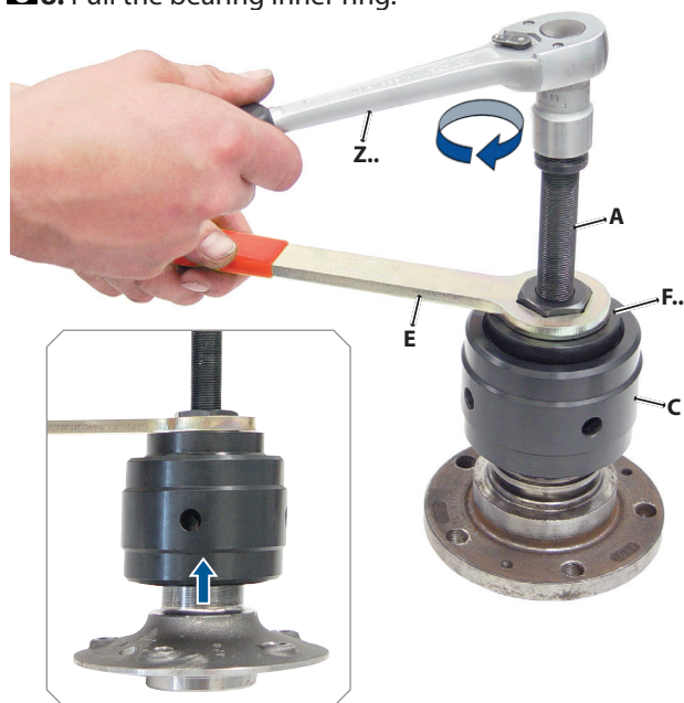
📸8: Pull the bearing inner ring.
