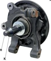
**9.** Depending on the wheel bearing **Ø**, select a suitable thrust ring **[P..]** which fits exactly on the inner ring on the wheel bearing.
