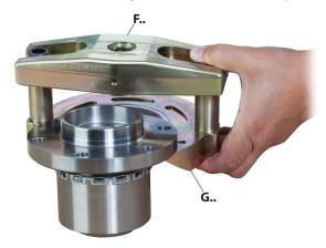
**1.** Place the bridge **[F..]** with the tension/pressure plate **[G..]** in the correct position on the new wheel bearing unit as shown.
