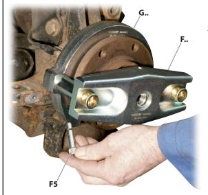
**3.** Place the bridge **[F..]** with tension/pressure plate **[G..]** in the correct position over the wheel bearing unit as shown.
