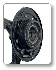
**6.** Check the correct installation position of the wheel bearing according to the manufacturer's specifications, remove the wheel bearing tool and, if necessary, insert the wheel bearing retaining ring on the steering knuckle.
