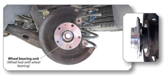
**7.** Check the correct installation position of the wheel bearing unit and reassemble the vehicle according to the manufacturer's instructions.
