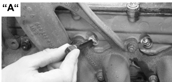
Fig. 2: Glow plug thread cleaning or repair.
