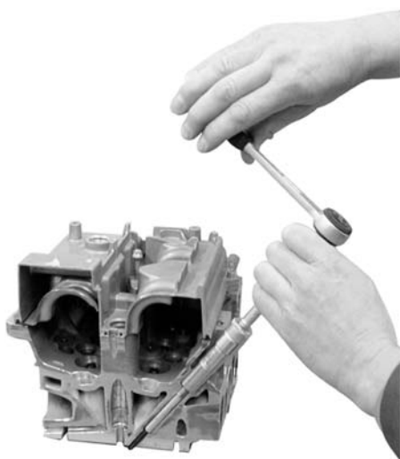
Fig. 1: Twisting off the glow plug top connector
