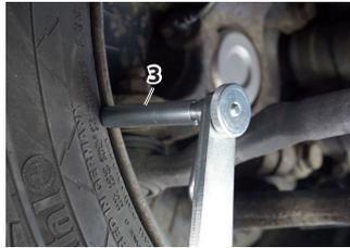
**Fig. 2:** Placing the toe measuring gauge between the wheels in front of the axle .
