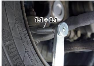
**B** When measuring on the **tyre**, use thrust pieces - **KL-0169-603**.
