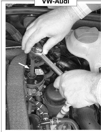
**KL-4021-3113 - Screwdriver Bit Socket, Size (waf) 13 mm**
