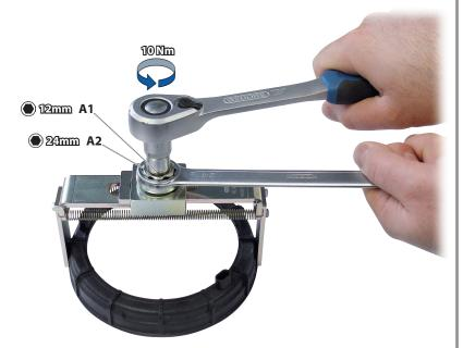
**6**4: Loosen or tighten the tank locking ring according to the <u>manufacturer's instructions</u>...
